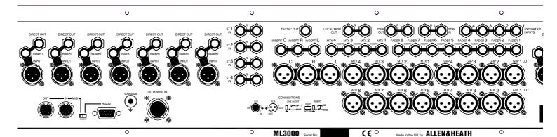
**CHANNEL INPUT** XLR input for mic or line level signals. Pin 2 hot. Phantom power is fed to pins 2 and 3 through 6k8 series resistors when the front panel +48V switch is pressed.
