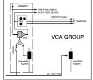
VCA groups affect the channel post-fade sends. They do not affect the pre-fade sends. Use VCA groups for level control. Use audio groups when you need to insert signal processing or feed the matrix.
