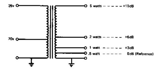
Figure 7-15. Details of a typical Distribution Transformer (JBL Model 9315HT)
