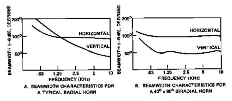
Figure 343. Increasing DI through Narrowing Vertical Beamwidth
