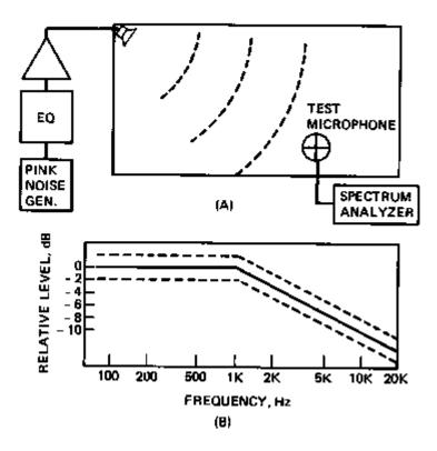
Figure 6-17. Sound System Equalization Procedure
