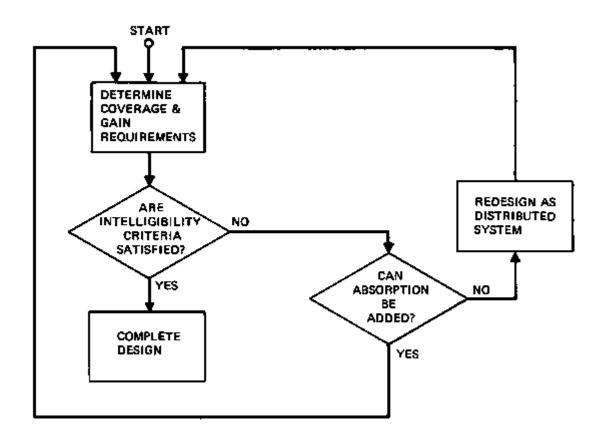
Figure 6-20. Flow Diagram for System Design
