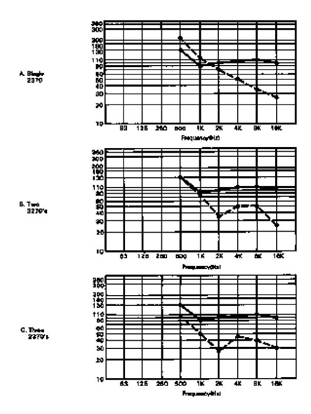
Figure 3-13. Stacking Horns for Higher Directivity at Low Frequencies (Solid Line, Horizontal -6 dB Beamwidth, Dashed Line, Vertical -6dB Beamwidth)
