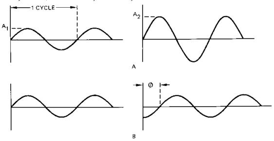
A - TWO SINE WAVES DIFFERING IN AMPLITUDE B - TWO SINE WAVES DIFFERING IN PHASE RELATIONSHIP
