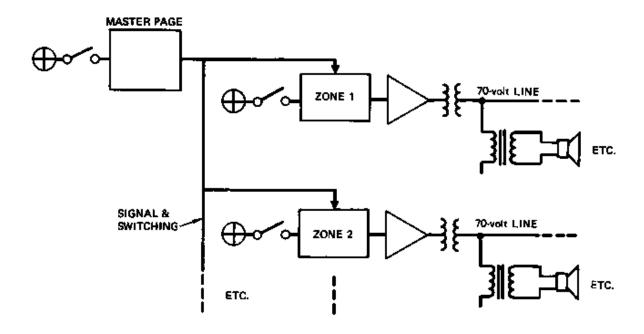
Figure 7-16. Block Diagram of a Paging System
