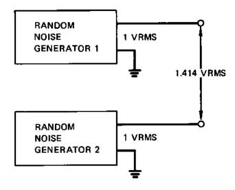
Figure 1-3. Combining Two Random Noise Generators
