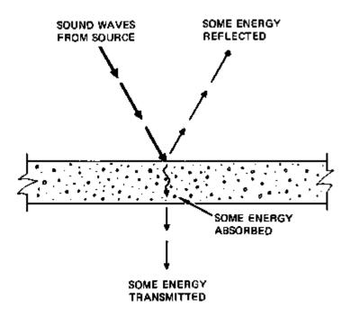
ALL THREE EFFECTS MAY VARY WITH FREQUENCY AND ANGLE OF INCIDENCE. THEY DO NOT VARY WITH INTENSITY IN TYPICAL SITUATIONS.
