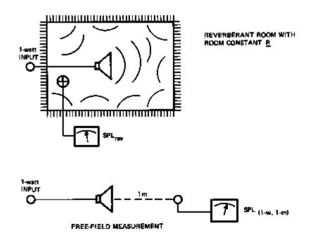
Figure 3-9: Reverberant Room Method for Measuring Directivity
