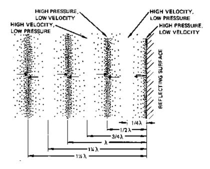
A PLANE WAVE REFLECTED FROM A PLANE SURFACE AT NORMAL INCIDENCE PRODUCES WELL-DEFINED ZONES OF HIGH PRESSURE ALTERNATING WITH ZONES OF HIGH PARTICLE VELOCITY AT DISTANCES OF ONE-QUARTER WAVELENGTH.
