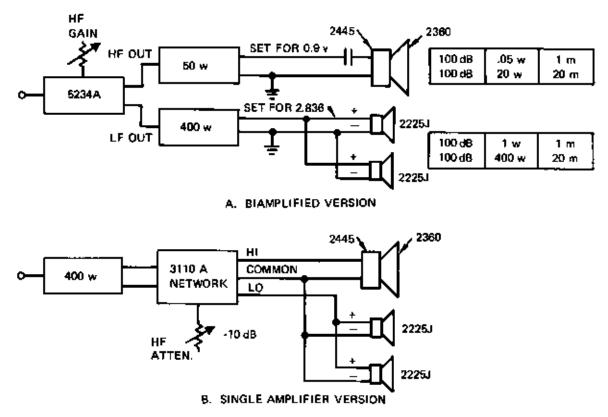
Figure 7-4. Matching HF and LF Components
