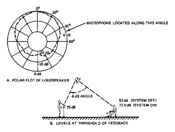
Figure 4-4. System Gain Calculations, Directional Loudspeaker
