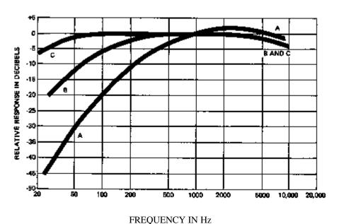
Figure 2-3. Frequency Responses for SLM Weighting Characteristics
