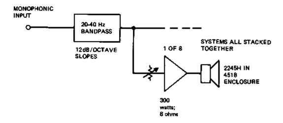
Figure 7-10. Implementation of a Sub-woofer System
