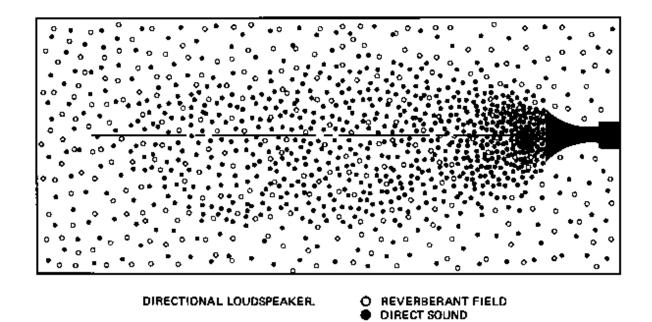
Figure 5-16. Direct and Reverberant Fields, Directional Loudspeaker
