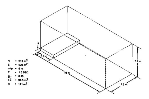
Figure 6-4. A Sound System in a Medium-Size Room
