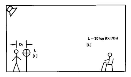
BRACKETS INDICATE LEVELS WITH SYSTEM ON.
