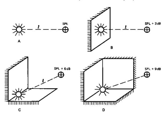
Figure 3-1. Directivity and Angular Coverage
