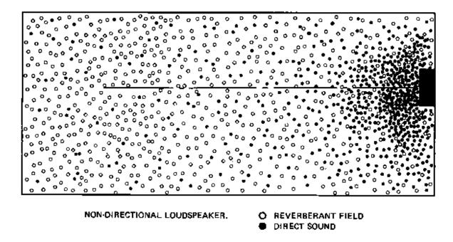
Figure 5-15. Direct and Reverberant Fields, Non-Directional Loudspeaker
