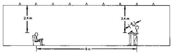
MIC, IS OMNIÐIRECTIONAL. SPKRS, PRODUCE EVEN SOUND FIELD AT EAR LEVEL.
