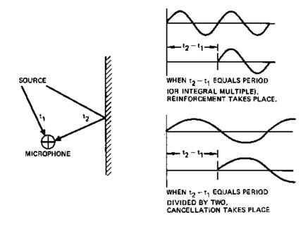
Figure 1-4A. Combining Delayed Signals
