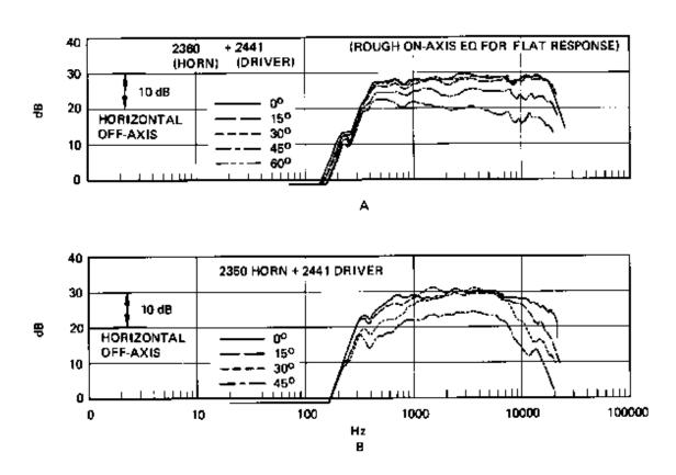
Figure 36. Families of Off-Axis Frequency Response Curves
