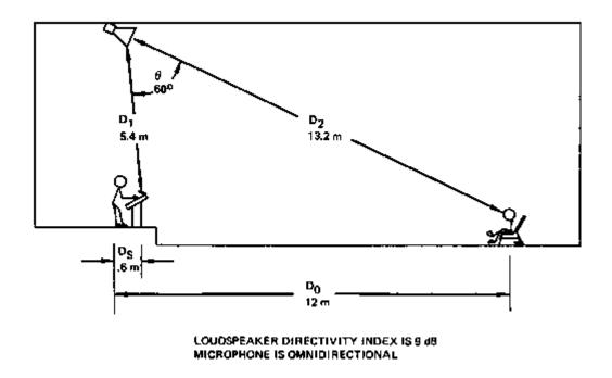
Figure 6-5. Sound System in a Medium-Size Room, Gain Calculations
