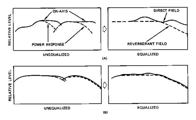
Figure 6-18. System Equalization
