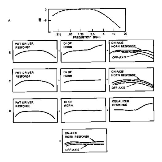
Figure 3-7. Power Response of HF Systems
