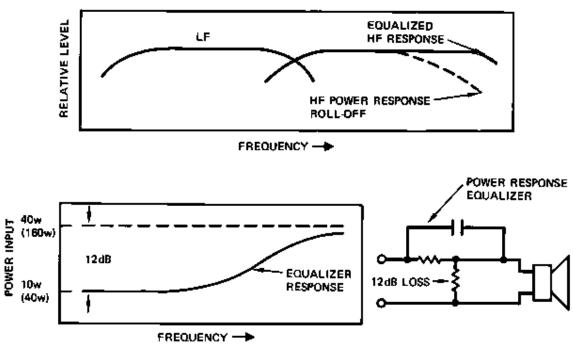
AT MID-FREQUENCIES, HF SECTION CAN BE DRIVEN WITH AS MUCH AS  $4\times40$ , OR 160 watts; HOWEVER, AT HIGH FREQUENCIES, 40 watts MAXIMUM MUST NOT BE EXCEEDED.
