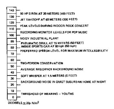
Figure 24. Typical A-Weighted Sound Levels
