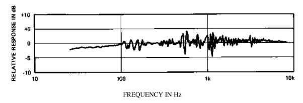
Figure 4-2. Electrical Response of a Sound System 3 dB Below Sustained Acoustical Feedback
