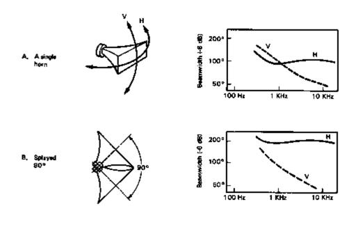
Figure 3-12. Horn Splaying for Wider Coverage
