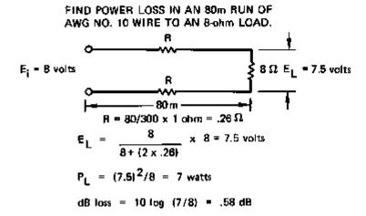
Figure 7-8. Resistance of Wire Runs
