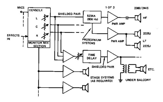
Figure 7-7. A Three-Channel Theater Reinforcement System
