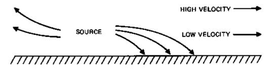
Figure 1-9. Effect of Wind Velocity Gradients on Sound Propagation
