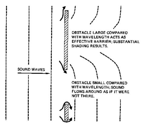
Figure 1-7. Diffraction of Sound Around Obstacles
