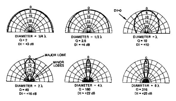
Figure 3-6. Directional Characteristics of a Circular-Piston Source Mounted in an Infinite Baffle as a Function of Diameter and  $\lambda$ .
