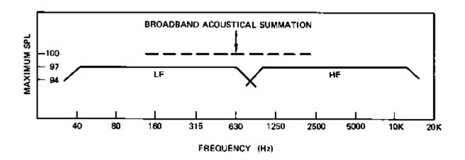
Figure 7-6. Acoustical Summation of HF and LF Sections
