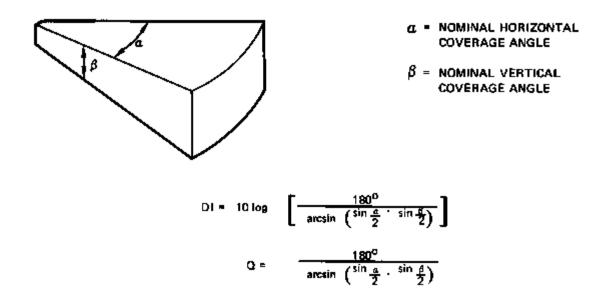
Figure 3-3. Illustration of Molloy's Equation
