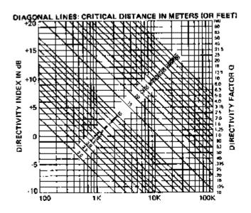
NOTE: EQUATIONS AND CHART CAN BE USED WITH ENGLISH OR METRIC UNITS. TO CONVERT CHART SCALES TO MORE CONVENIENT VALUES FOR METRIC CALCULATIONS, DIVIDE CRITICAL DISTANCES BY 10 AND ROOM CONSTANTS BY 100.
