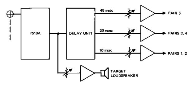
Figure 7-13. Block Diagram, Church Distributed System
