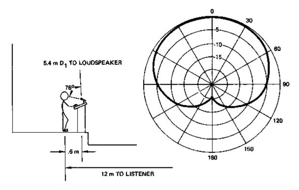
Figure 6-7. Characteristics of a Cardioid Microphone
