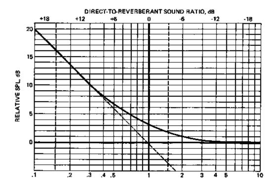
RATIO OF DISTANCE FROM THE SOURCE TO CRITICAL DISTANCE CALCULATED FROM:  $10 \log(1+1/x^2)$  WHERE x IS THE RATIO OF DISTANCE FROM SOURCE TO CRITICAL DISTANCE
