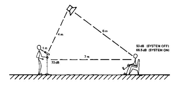
Figure 4-3. System Gain Calculations, Loudspeaker and Microphone Omnidirectional
