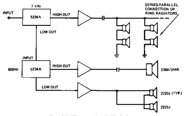
Figure 7-19. HF Augmentation with Ring Radiators
