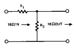
USE ADJUSTABLE WIRE-WOUND RESISTORS OF ADEQUATE POWER RATING.
