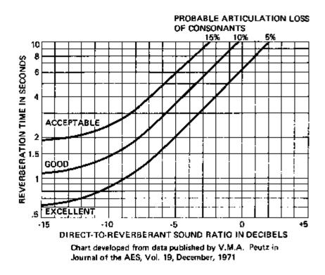
Figure 6-13. Probable Intelligibility as a Function of Reverberation Time and Direct-to-Reverberant Sound Ratio
