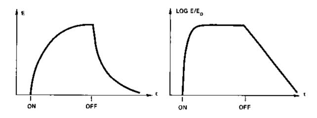
Figure 5-6. Idealized Growth and Decay of Sound Energy in an Enclosure
