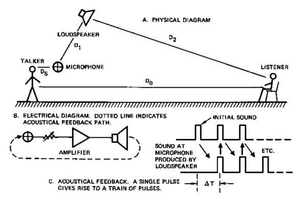
Figure 4-1. A Simple Outdoor Reinforcement System
