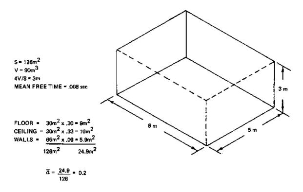
Figure 5-8. Calculating Reverberation Time
