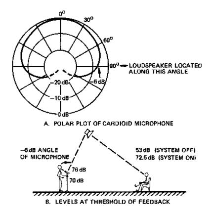
Figure 4-5. System Gain Calculations, Directional Microphone
