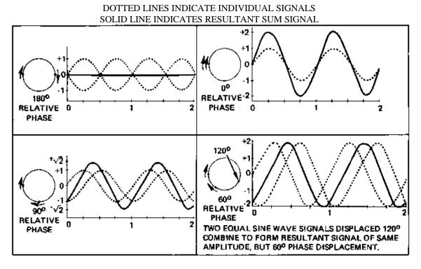
Figure 1-2. Vector Addition of Two Sine Waves
