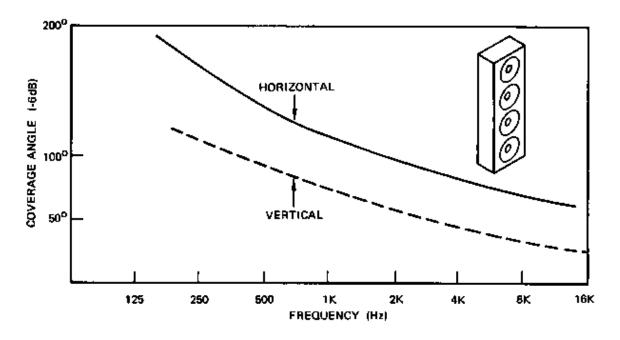
Figure 7-12. Directivity Characteristics of a Sound Column
