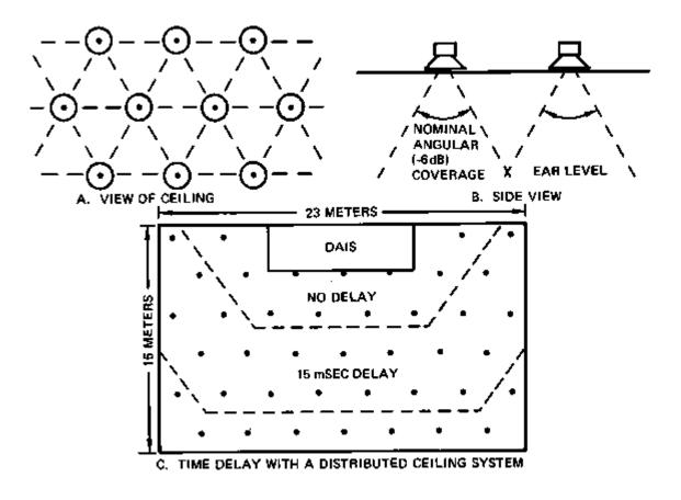
Figure 7-17. Ceiling Lay-out of Distributed Loudspeakers
