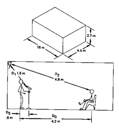
Figure 6-2. Indoor Sound System Gain Calculations
